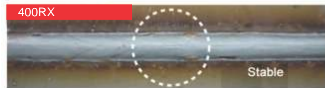
Welding seam comparison as input voltage varies
